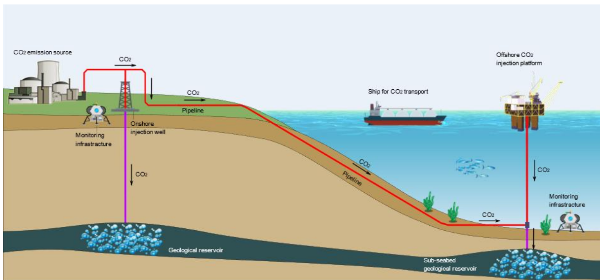
Figure 3: Key elements and processes in offshore CCUS. Offshore CCUS captures CO 2 from industrial emission sources, transports it via either pipeline or ship, and injects it into sub-seabed geological reservoirs, contributing to the isolation of CO 2 from the atmosphere.
