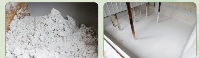
Figure 5. Brine sludge waste (Credit: Fuhua Tongda Chemical Co., Ltd.)
